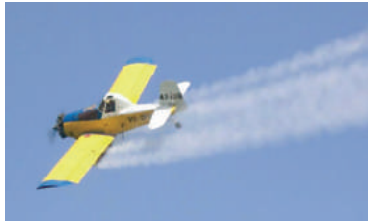
Cloud seeding aircraft using salt powder
